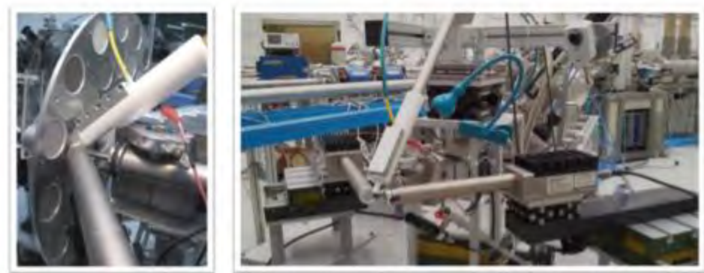
Fig.1 – The PIXE setup at the INFN-LABEC laboratory allows very sensitive and rapid (1 minute/sample) measurements of all the main crustal elements, thus making this technique a very effective tool to assess the actual impact of Saharan dust episodes.
